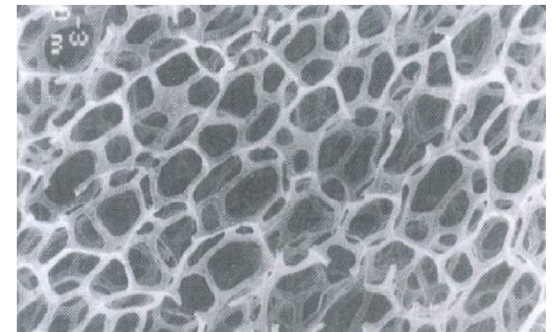
Magnified Image Open Celled Foam, Acoustics
